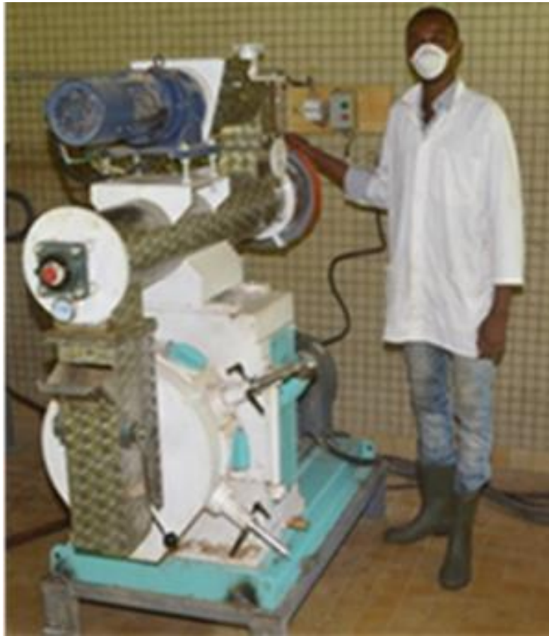
Figure 18: Existing pelletizing mill in Côte d'Ivoire, to be replaced with a higher throughput mill to increase viability of animal feed pellet production
