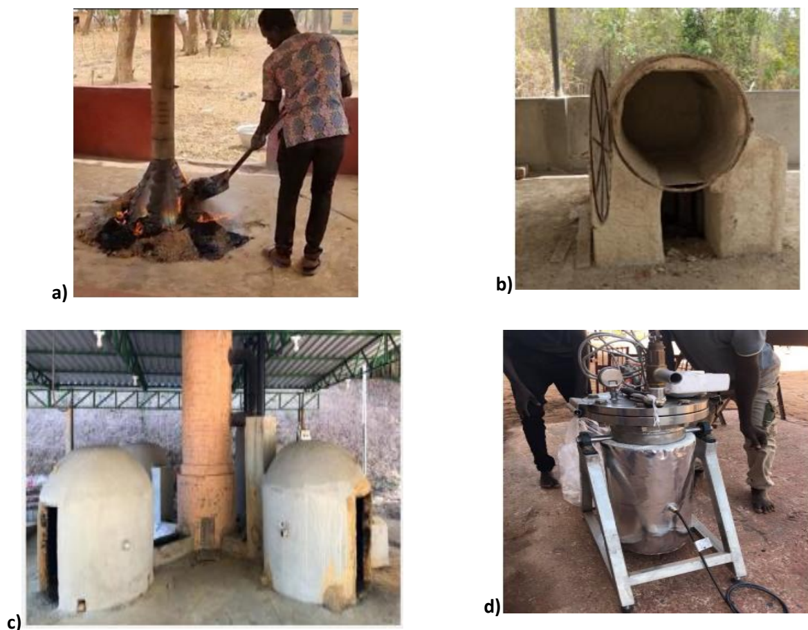
Figure 9: Carbonisation technologies in the BIO4AFRICA project using traditional kilns, e.g. kilns from a) Ghana and b) Côte d'Ivoire; adapted, pollution-reducing kilns, e.g. wood-burning kilns from Brazil (c); and hydrothermal carbonization technology, e.g. as adapted for use in Senegal (d).
