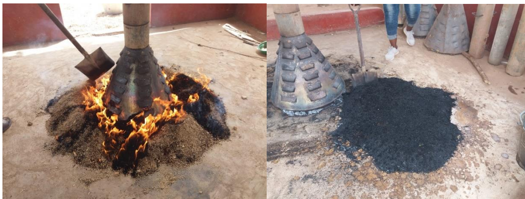
Figure 12: Pictures of biochar production using local pyrolysis technology in Ghana
