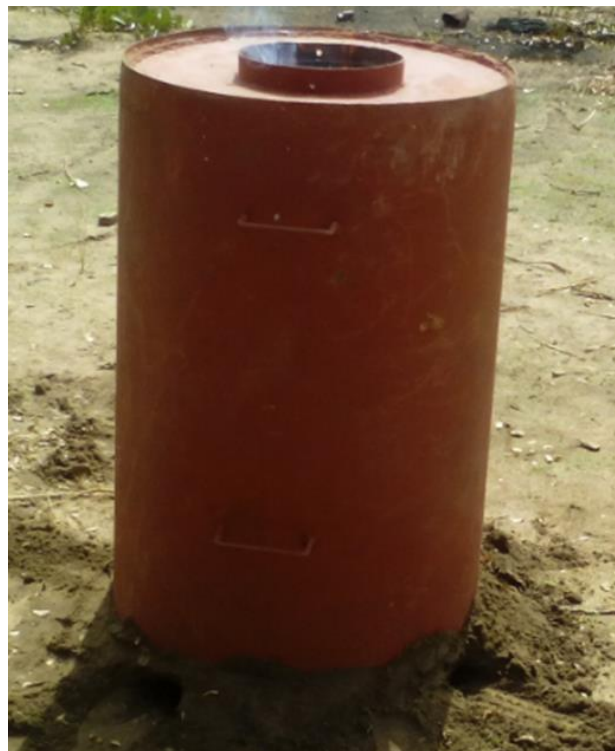
Figure 8: Kilns manufactured from standard 45 gallon oil drums, Zinguinchor, Senegal
