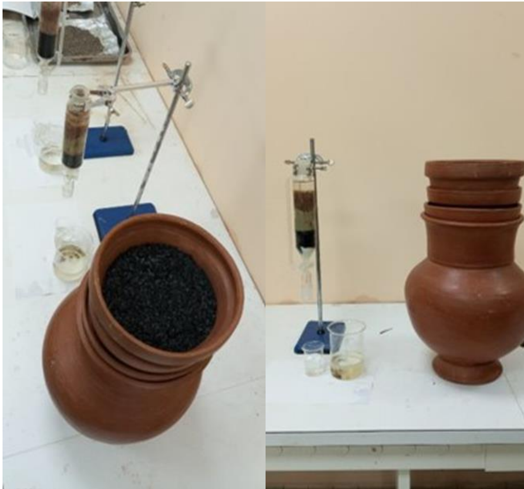
Figure 21 : Laboratory device using Biochar as water filter, INP-HB, Côte d'Ivoire
