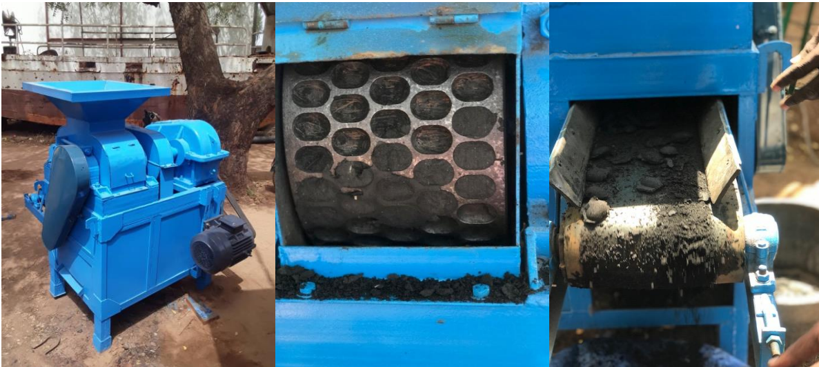
Figure 20: Photos of briquetting line to be piloted in Senegal for biochar briquetting pilot activities
