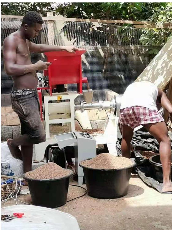
Figure 17: Pilot scale pelletization technology in Ghana
