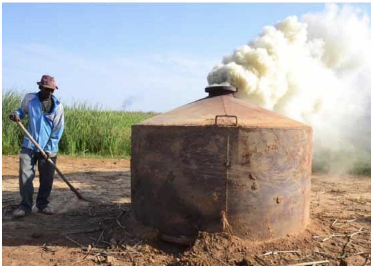
Figure 9: Cylindrical transportable metal kilns for charcoal production, Zinguinchor, Senegal
