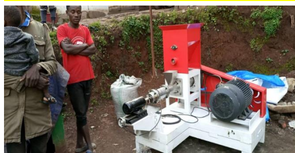
Figure 17: Pilot scale pelletization technology in Ghana
